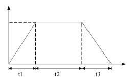
Figure 4-8 Jog Frequency Diagram
