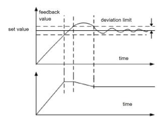
Fig.4-19 diviation limit schematic
