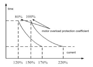
Fig. 4-27 Motor's overload protection efficient setting. protection efficient is decided by the following formula:
