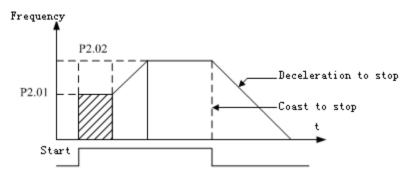
Figure 45 Starting and Stopping Diagram
