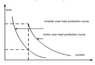
Fig. 4-26 inverter's overload protection and motor's overload protection curve
