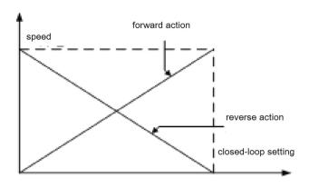
Fig.4-18 forward/reverse characteristics illustration
