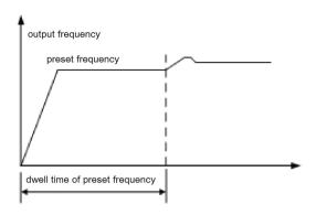
Fig.4-20 closed-loop preset frequency operation schematic
