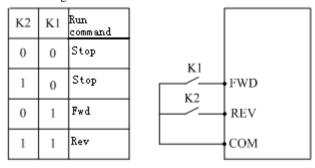
Figure 4-11 2-Wire Control Mode 2
