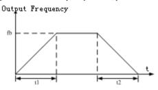
Figure 43 Acceleration and Deceleration time
