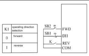
Fig.4-13 3-wire type control mode 2
