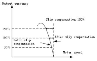
Figure 42 Slip Frequency Compensation Diagram
