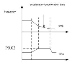
Fig.4-28 overload restriction level illustartion.
