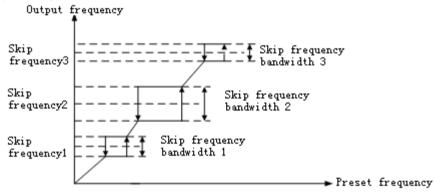
Figure 49 Skip Frequency Diagram
