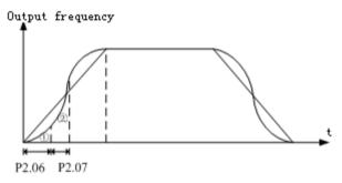
Figure 46 S Curve Diagram
