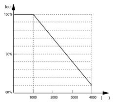
Fig. 1-3 derating usage illustration of inverter's rated output current and altitude  $1.4\ \mathrm{Protection}\ \mathrm{Level}$
