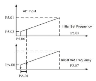
Fig 4-29 Zero frequency retrun difference operation
