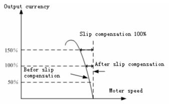
Figure 6-2 Slip Frequency Compensation Diagram
