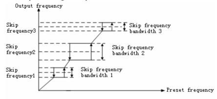
Figure 6-10 Skip Frequency Diagram
