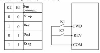
Figure 6-11 2-Wire Control Mode 1
