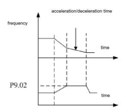
Fig. 6-32 overload restriction level illustartion.
