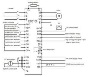
Fig.3-5 Basic Running Wiring Diagram
