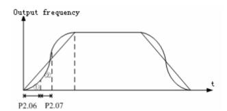
Figure 6-7 S Curve Diagram
