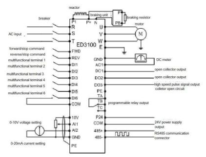
Form 3-6 Basic Running Wiring Diagram  $\,$  FIT MODELS: ED3100-4T0220M $\sim$  ED3100-4T4000M  $\,$
