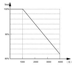
Fig. 1-4 derating usage illustration of inverter's rated
