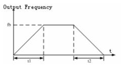
Figure 6-3 Acceleration and Deceleration time
