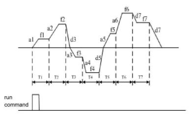
Fig.6-26 single cycle schematic
