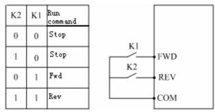
Figure 6-12 2-Wire Control Mode 2
