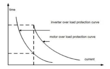
Fig. 6-30 inverter's overload protection and motor's overload protection curve
