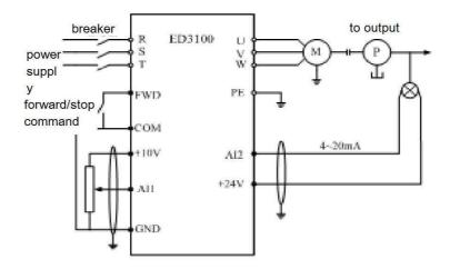
Fig.6-20 analog feedback control system schematic
