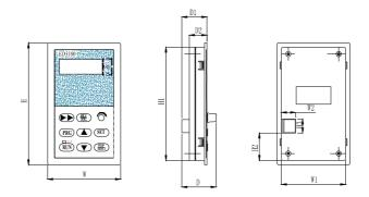
ED3100-RKD Remote Control Keyboard SPEC. Form 2-3 ED3100 ED3100 remote control keyboard outline and installation dimensions.
