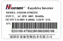
Fig. 1-2 Inverter Nameplate
