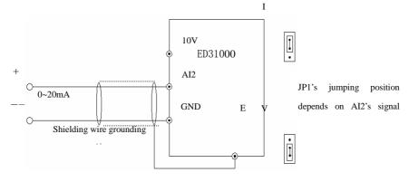
Fig. 3-9 AI2 terminal wiring
