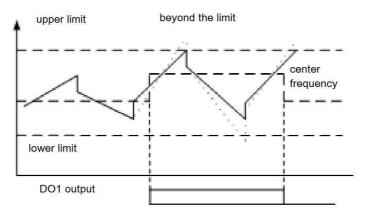
Fig 6-15 transverse operation upper and lower limit schematic **15:** programmable multi-step speed staged operation ends.
