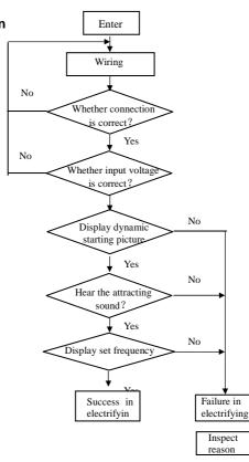
Diagram 4-4 Flow chart of inverter initially electrified operation
