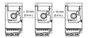
Free space  $\geq$  10 mm (0.4 in.) on each side, with vent cover fitted. Mounting type A is suitable for drive operation at surrounding air temperatures less than or equal to 55°C.
