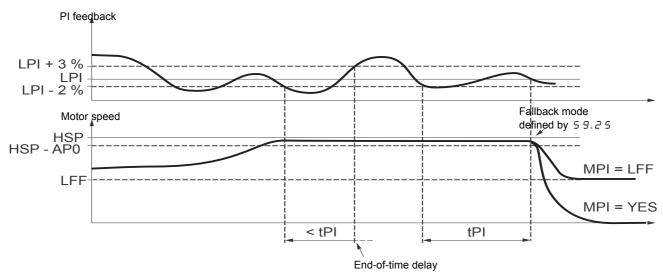
Once the variable pump is running at maximum speed (higher than  $5 \ l \ 2 \ 2 - 5 \ 9 \ 2 \ 4$ ) and at the same time the PI feedback is lower than the supervision threshold  $5 \ 9 \ 2 \ 2 - 2\%$ , a time delay tPI is launched. If at the end of this time delay the value of the PI feedback is still lower than the supervision threshold  $5 \ 9 \ 2 \ 2 + 3\%$ , the drive switches to fallback mode as defined by parameter  $5 \ 9 \ 2 \ 5$ .
