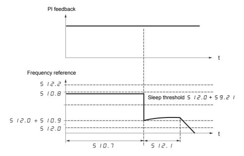
• Set the sleep function so that the drive switches to sleep mode when zero flow is detected (5 9.2 / ≤ 5 9.2 /).
