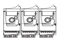
Drives mounted side-by-side with vent covers removed. Mounting type B is suitable for drive operation at surrounding air temperatures less than or equal to  $55^{\circ}$ C.
