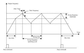
Fig.6-25 swing frequency operation Diagram
