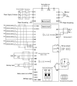
Fig.3-3-2 Terminal Wiring (Type 2R2GB-4R0GB as Example)
