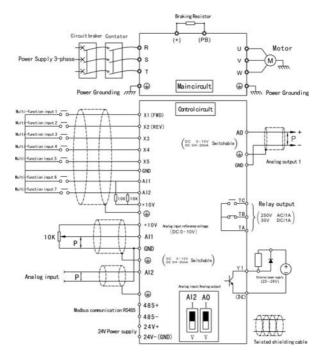
Fig.3-3-1 Terminal Wiring (Type 0R4GB-1R5GB as example)
