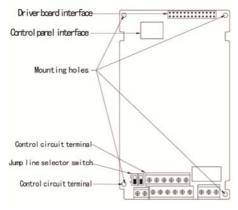
Fig.3-10 Control board schematic drawing
