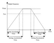
Fig.6-2 Schematic diagram for acceleration/deceleration time
