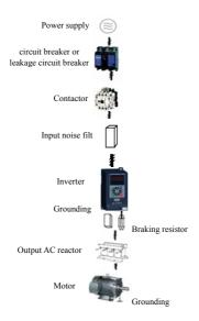
Fig.3-1 Connection diagram of the product and peripheral devices
