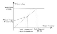
Fig.6-10 Schematic Diagram for Manual Torque Boost
