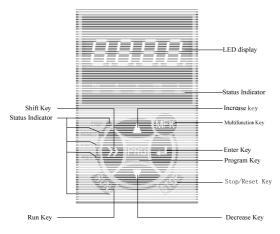
Fig.4-1 Operation Panel Diagram
