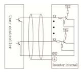
Fig.3-6 NPN common emitter wiring mode
