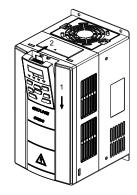
Fig. 3-3 Remove keypad
