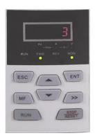
Fig. 4-10 Second-tier display of parameter ("3" is the value of b0-00)
