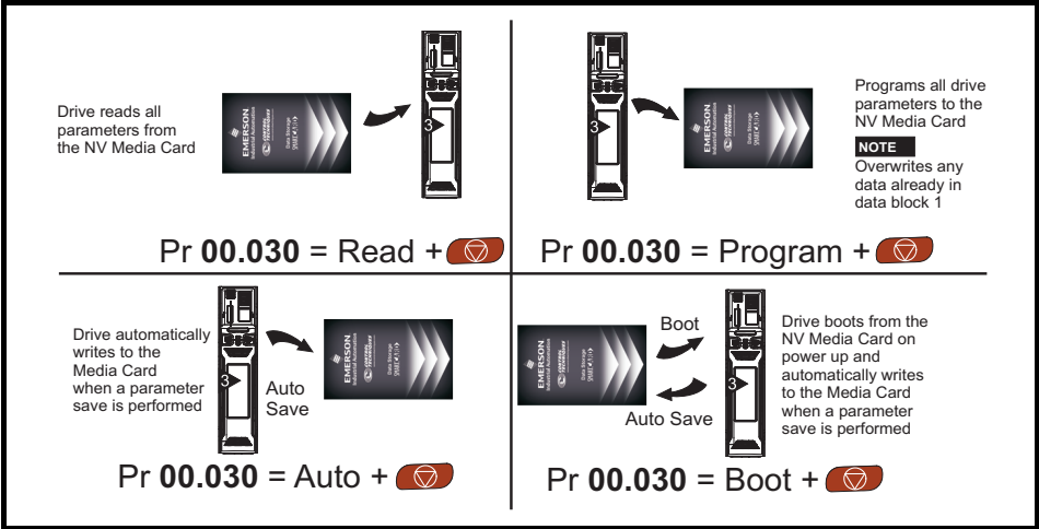
Figure 8-2 Basic NV Media Card operation
