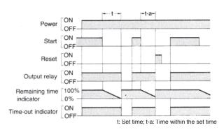
Note: 1. The minimum signal input time is 0.05 s.
