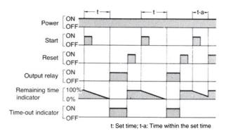
Note: The minimum signal input time is 0.05 s.
