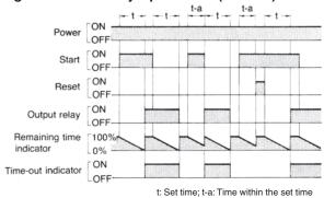
Signal ON/OFF-delay Operation 2 (H Mode)
