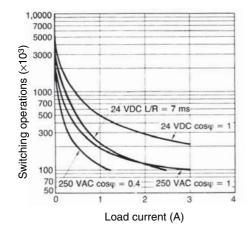
Reference: A maximum current of 0.15 A can be switched at 125 VDC ( $\cos \phi = 1$ ). Maximum current of 0.1 A can be switched if L/R is 7 ms. In both cases, a life of 100,000 operations can be expected.
