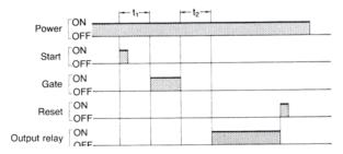
**Note:** 1. This timing chart indicates the gate input in operation mode A (ON-delay operation).
