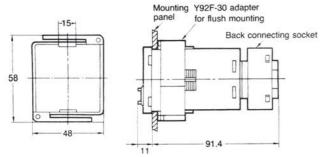
**Note:** Pay attention to the orientation of the adapter when mounting two or more timers in a vertical or horizontal line.
