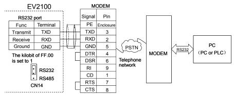
Fig. 3-19 Wiring of RS232-(MODEM-PSTN-MODEM)-RS232 communication
