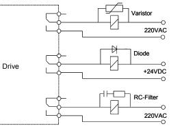
Fig. 3-41 Relay, contactor and electro-magnetic braking kit
