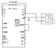
Fig. 7-1 Insulation test of drive
