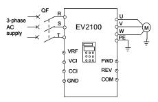
Fig. 3-7 Wiring
