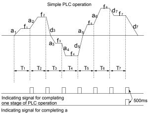
Indicating signal for completing cycle of PLC operation
