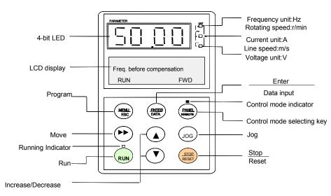
Fig. 4-2 Illustration of operation panel
