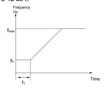
Fig. 5-12 Starting frequency and starting time
