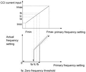
fa: Zero frequency threshold fb: fa+ zero freq. hysteresis fc: Freq. corresponding to Ic(CCI input)
