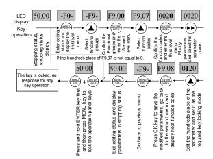
Fig. 4-14 Operation example for unlocking the operation panel keys
