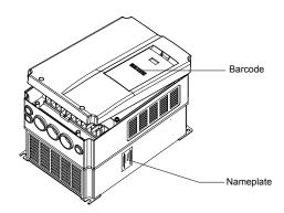
Fig. A-2 Locations of Nameplate and Barcode
