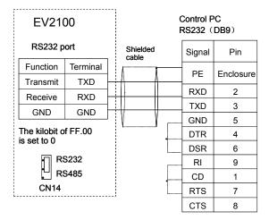
Fig. 3-17 RS232-RS232 communication cables
