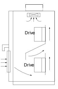
Fig. 3-3 Installation of several drives
