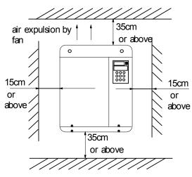
Fig. 3-2 Installation clearance (75kW or above)
