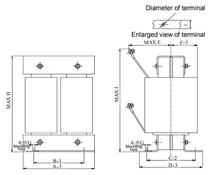
Fig. 2-3 Dimensions of DC reactor
