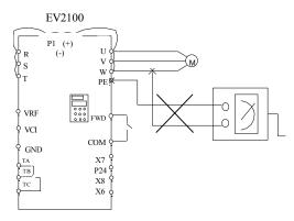
Fig. 7-2 Insulation test of motor
