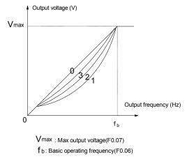
Fig. 5-5 Torque-reducing curve
