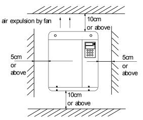
Fig. 3-1 Installation clearance (55kW or below)
