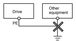
Fig. 3-39 Earthing diagram 3
