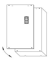
Fig. 3-6 Removing and mounting metal cover
