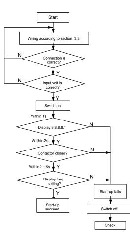
Fig. 4-16 Procedures of first time drive start up
