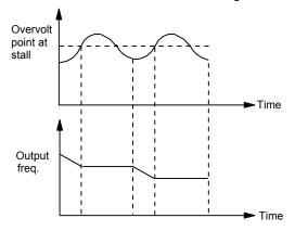
Fig. 5-63 Over-voltage at stall
