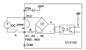
Fig. 3-23 Using an external supply
