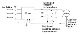
Fig. 3-42 Flowing path of leakage current
