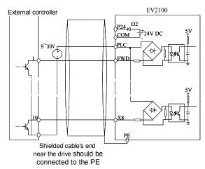
Fig. 3-26 Method 2 of connections(c)
