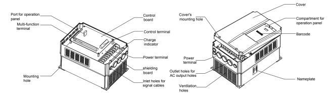
Fig. 2-1 Structure of drive
