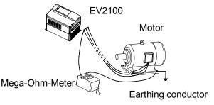
Fig. 1-1 Checking the insulation of motor
