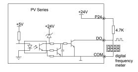
Fig. 3-29 Wire connections 1 of output terminal DO
