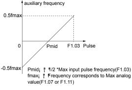
Fig. 5-52 Using PULSE-0.5×F1.03 to determine auxiliary reference frequency
