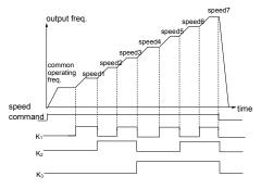
Fig. 5-29 Multi-step speed operation
