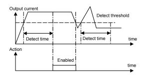
Fig. 5-63 Overload pre-alarm function
