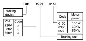
Fig. 2-6 Model of braking unit
