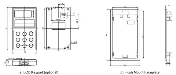
Fig. 2-4 Operation Keypad and flush mount faceplate
