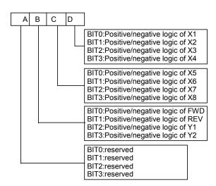
Fig. 5-41 terminal's positive and negative logic
