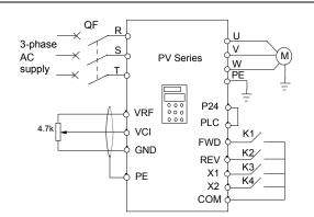
Fig. 5-48 Wiring connections for remote and local control
