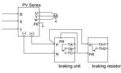
Fig. 2-10 Connecting the braking unit to Drive
