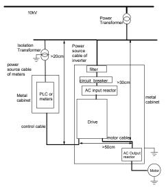
Fig. 3-43 Installation of the drive
