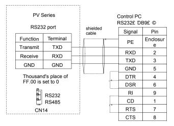
Fig. 3-16 RS232-RS232 communication cables
