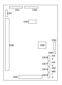
Fig. 3-11 Locations of jumpers on the control board
