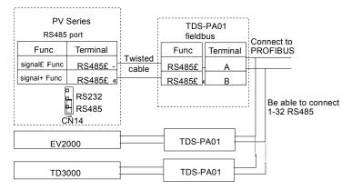
④ The drive's RS485 port connects to PROFIBUS-DP via the TDS-PA01(made by ENPC):
