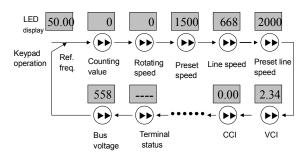
Fig. 4-7 Display parameters in running status
