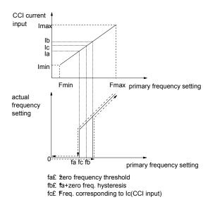
Fig. 5-57 Hysteresis of zero-frequency operation
