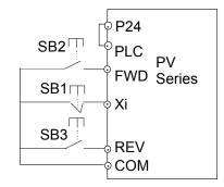
Fig. 5-34 3-wire operating mode 1 Where:
