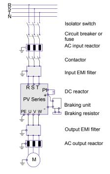
Fig. 3-8 Wire connection between the drive and optional parts
