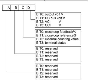
Fig. 5-43 Operating parameter 2 displayed by LED
