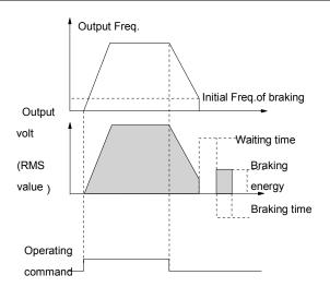
Fig. 5-13 Dec-to-stop + DC injection braking
