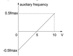
fmax; † frequency corresponding to Max analog value(F1.07 orF1.11)
