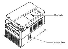
Fig. A-3 Locations of Nameplate and Barcode
