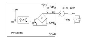
Fig. 3-28 Wire connections 2 of multi-function output terminal
