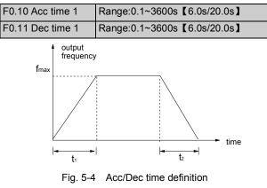
Acceleration time is the time taken for the motor to accelerate from 0Hz to the maximum frequency (as set in F0.05), see  $t_1$  in Fig. 5-4.
