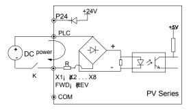
Fig. 3-22 Wire connections when an external power supply is used
