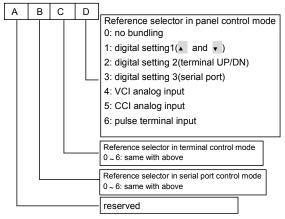
Fig. 5-46 Control mode is bundled to frequency selector
