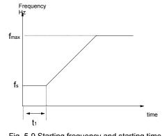
Fig. 5-9 Starting frequency and starting time
