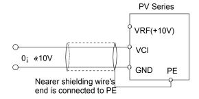
Fig. 3-13 Wire connections for terminal VCI
