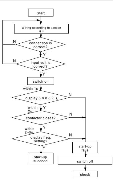
Fig. 4-16 Procedures of starting the drive for the first-time
