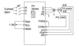
Fig. 5-22 Wiring diagram of Speed close-loop with PG
