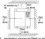
Fig. 3-2 Installation clearance(75kW or above)
