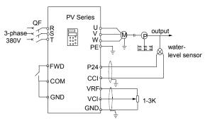
Fig. 5-21 Analog feedback control system with internal PI
