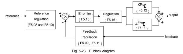
In the above Figure, KP: proportional gain; Ki: Integral gain, refer to F5.01~F5.15 for the definitions of close-loop reference, feedback, error limit and proportional and Integral parameters.
