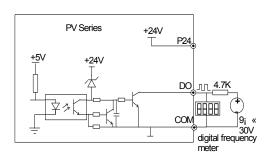
Fig. 3-30 Wire connections 2 of output terminal DO
