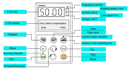
Fig. 4-2 Illustration of operation panel
