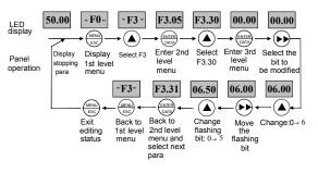
Fig. 4-8 Example of setting the parameters
