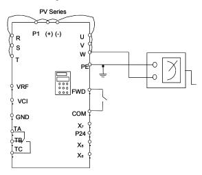
Fig. 7-1 Insulation test of drive
