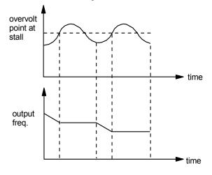
Fig. 5-61 Over voltage at stall
