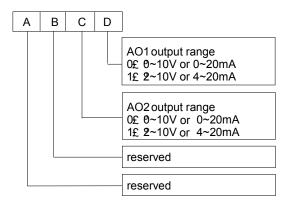
Fig. 5-39 analog output offset settings
