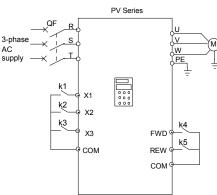
Fig. 5-30 Wiring for multi-speed operation
