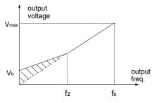
Vb£ fnanual torque boost Vmax£ Max output voltage fz£ cut-off freq. for torque boost fb£ basic operating freq.
