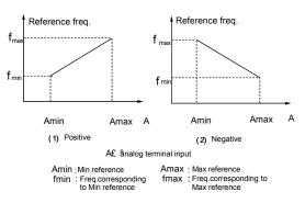
Fig. 5-8 Output frequency curve
