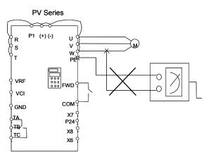
Fig. 7-2 Insulation test of motor
