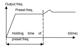
Fig. 5-28 Preset frequency of close-loop operation
