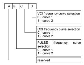
Fig. 5-9 Frequency curve selection
