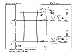
Fig. 3-23 Connection method 2 (a)
