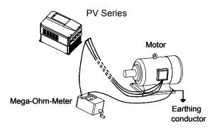
Fig. 1-1 Checking the insulation of motor
