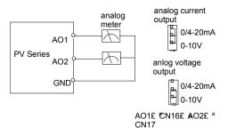
Fig. 3-15 Wire connections for analog output terminal
