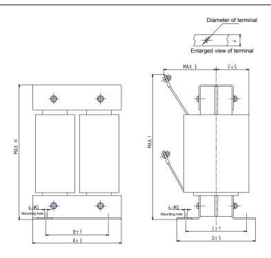
Fig. 2-3 Dimensions of DC reactor
