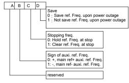
Fig. 5-53 digital auxiliary reference frequency control Where.
