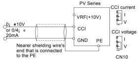
Fig. 3-14 Wire connections CCI
