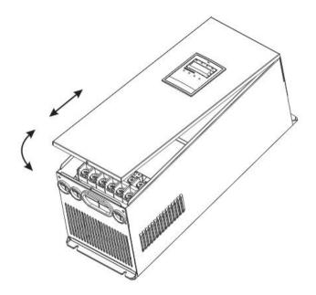
Figure 3.4 Disassembly of cover.
