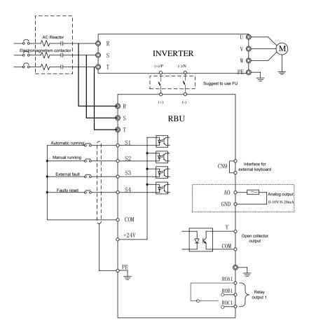
Figure 4.3 Wiring Diagram.
