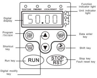
Figure 5.1 Keypad schematic diagram.
