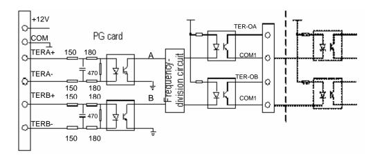
Figure 3.4 Wiring diagram of frequency-division output.
