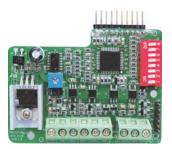
Option card for CHV series close loop vector control inverter
