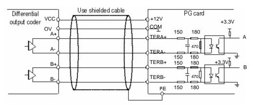
Figure 3.1 Wiring diagram of differential output
