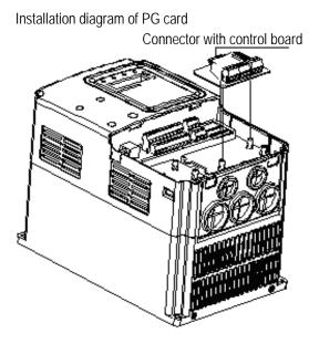
Figure 1.1 Installation of PG card
