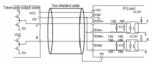
Figure 3.3 Wiring diagram of push-pull output
