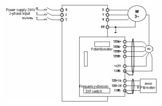
Figure 2.2 Wiring Diagram.
