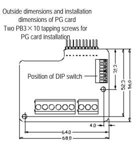
Figure 1.2 Dimensions of PG Card.
