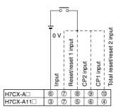
Operates when the contact turns  $\ensuremath{\mathsf{ON}}$ .
