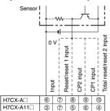
Operates when the transistor turns ON
