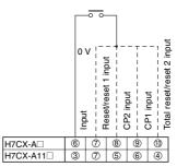
Operates when the contact turns ON.
