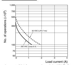
Reference: A current of 0.15 A max. can be switched at 125 VDC (coso=1) and current of 0.1 A max. can be switched if L/R=7 ms. In both cases, a life of 100,000 operations can be expected. The minimum applicable load is 10 mA at 5 VDC (failure level: P).
