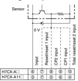
Operates when the transistor turns ON.
