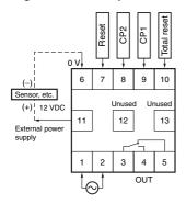
H7CX-AS/-A4S 1-stage Transistor Output
