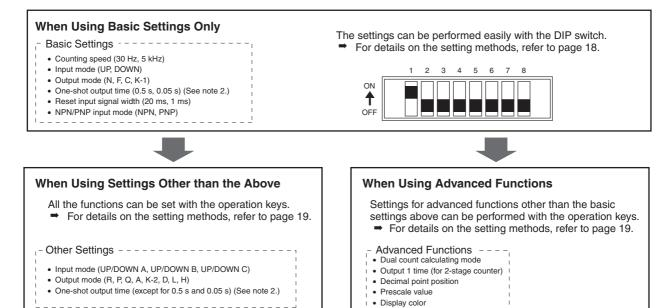
Note: 1. At the time of delivery, the H7CX is set to the 1-stage counter (2-stage counter for H7CX-AW\(\sigma\)/-A4W\(\sigma\) models) configuration.
