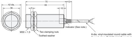
Note: D Models: Operation indicator (red), setting indicator (green) B, C, Y Model: Operation indicator (red) 2 conductors (D, Y Models)/3 conductors (B, C Models) (Conductor cross section: 0.5 mm², Insulator diameter: 1.9 mm), Standard length: 2 m The cable can be extended up to 200 m (separate metal conduit).
