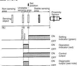
Note: The diagnostic output of the E2E-X□D1S is ON when there is a coil burnout or the sensing object is located in the unstable sensing range for 0.3 s or more.
