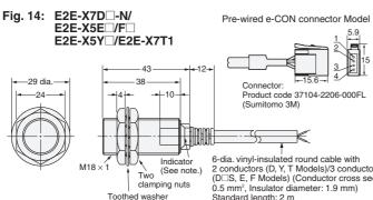
Note: D, T Models: Operation indicator (red), setting indicator (green); E, F, Y Models: Operation indicator (red)
