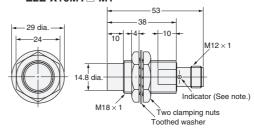
Note: D Models: Operation indicator (red), setting indicator (green) E, F, Y Model: Operation indicator (red)
