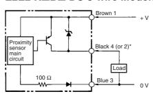
\* Pin 4 is an NO contact, and pin 2 is an NC contact.
