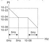
Ш When using multi-function input terminals to switch ASR1/ASR2, the diagram will be shown as follows.
