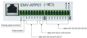
When wiring, please refer to the multi-function input/output function in parameters group 02 and group 03 of chapter 4 parameters to set by your applications.
