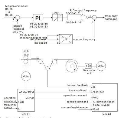
Line speed closed-loop, speed mode
