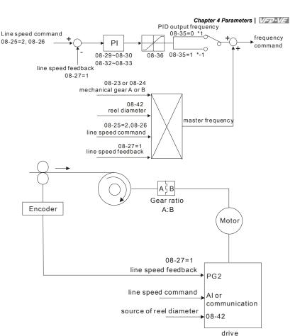
Tension open-loop, torque mode
