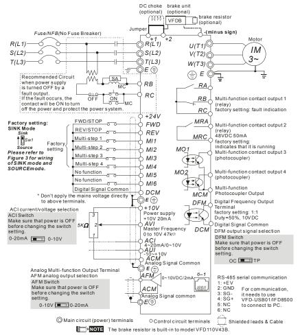
Figure 3 Wiring for SINK(NPN) mode and SOURCE(PNP) mode
