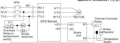
Note1: When using the AC drive with DC reactor, please refer to wiring diagram in the AC drive user manual for the wiring of terminal +(P) of Brake unit.
