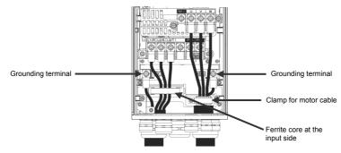
Figure 8.1 Wiring to Main Circuit Terminals for Inverters of 30/37 kW
