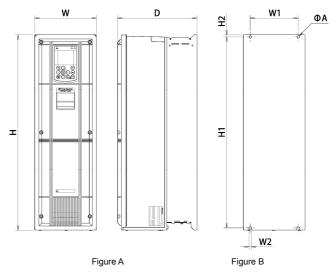
External Dimensions of the Inverter (Typical)
