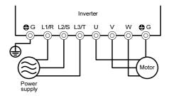
Figure 4.1 Connection of Main Circuit Terminals
