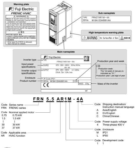
Note In this manual, inverter types are denoted as "FRN\_ \_\_AR1■-4□." The boxes ■ and □ replace alphabetic letters depending on the enclosure and shipping destination, respectively.
