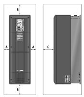
Figure 2.1 Mounting Direction and Required Clearances
