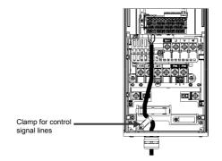
Figure 8.2 Wiring to Control Circuit Terminals for Inverters of 30/37 kW
