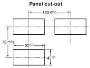
Mounting Recommended Panel Thickness 1 to 8 mm.
