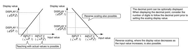
Instead of setting by inputting with the ② Up Key and ③ Shift Key, current values can be input as scaling input values for teaching. This is useful for making settings while checking the operation status of the K3MA-J.
