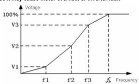
Figure 6.12 V/F curve setting diagram.
