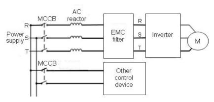
Figure 4.9 Wiring at input side.
