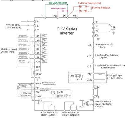
Figure 4. 8 Wiring diagram.
