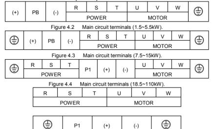
Figure 4.5 Main circuit terminals (132~315kW).
