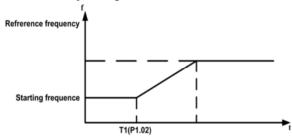
Figure 6.4 Starting diagram.
