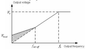
Figure 6.11 Torque boost diagram.
