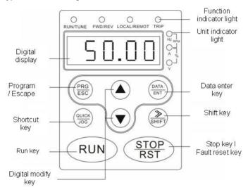
Figure 5.1 Keypad schematic diagram.
