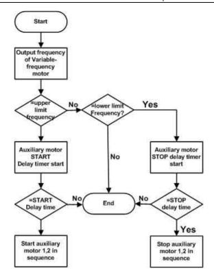
Figure 6.26 Simple water-supply function logical diagram.
