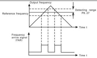
Figure 6.24 Frequency arriving detection diagram.
