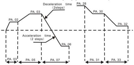
Figure 6.32 Simple PLC operation diagram.
