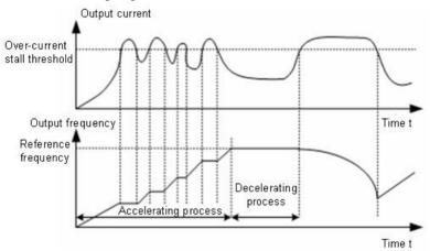
Figure 6.37 Over-current stall function.
