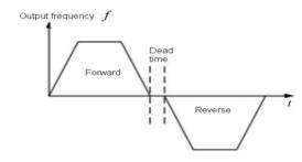
Figure 6.7 FWD/REV dead time diagram.
