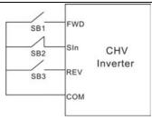
Figure 6.16 3-wire control mode 2.
