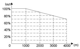
Figure 3.1 Relationship between output current and altitude.
