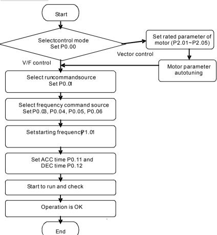
Figure 5.4 Quick start diagram
