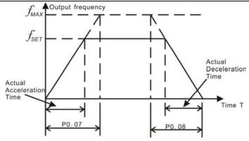
Figure 6.2 Acceleration and Deceleration time.
