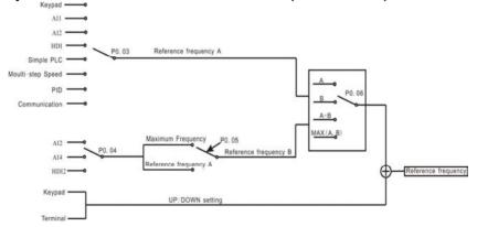
Figure 6.1 Reference frequency diagram.
