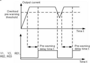
Figure 6.35 Overload pre-warning schematic diagram.
