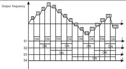
Figure 6.33 Multi-steps speed operation diagram.
