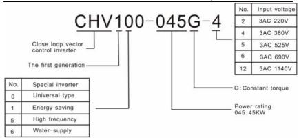
Figure 1.1 Nameplate of inverter.
