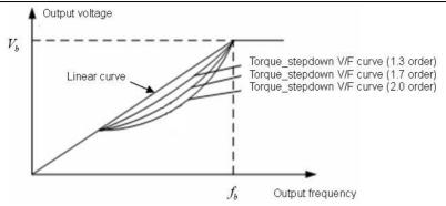
Figure 6.10 Multiple V/F curve diagram.
