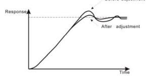
Figure 6.29 Reducing long-cycle oscillation diagram.
