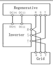
Figure 4.11 Wiring of regenerative unit.
