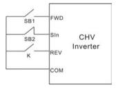
Figure 6.15 3-wire control mode 1.
