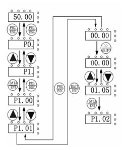
Figure 5.2 Flow chart of parameter setting.
