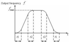
Figure 6.5 S curve diagram.
