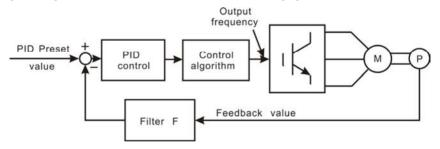
Figure 6.27 PID control diagram.
