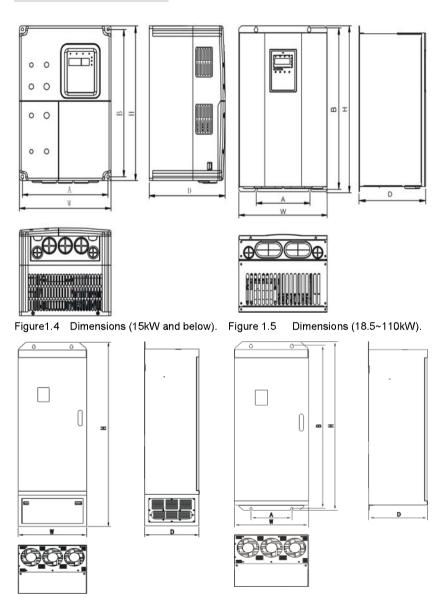
Figure 1.6 Dimensions (132~315kW).
