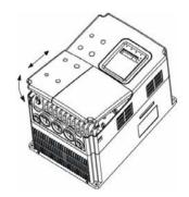
Figure 3.6 Disassembly of plastic cover.
