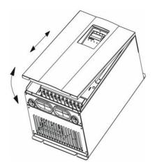
Figure 3.7 Disassembly of metal plate cover.
