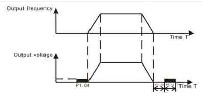
Figure 6.6 DC braking diagram.
