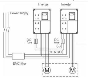
Figure 4.12 Wiring of common DC bus.
