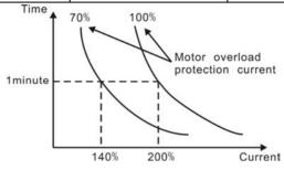
Figure 6.34 Motor overload protection curve.
