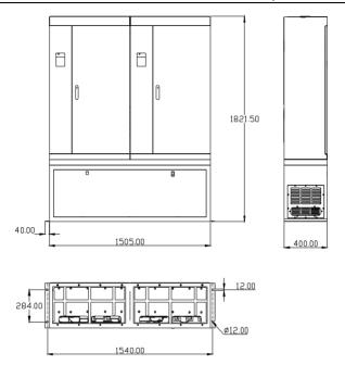
Figure 1.7 Dimensions (350kw~500W).
