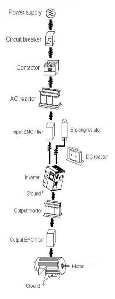
Figure 4.1 Connections of peripheral devices.
