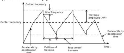
Figure 6.21 Traverse operation diagram.
