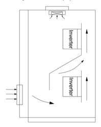
Figure 3.3 Installation of multiple inverters.
