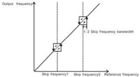
Figure 6.20 Skip frequency diagram.
