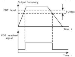
Figure 6.23 FDT Level diagram.
