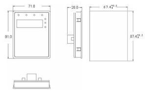
Figure 3.4 Dimensions of small keypad.
