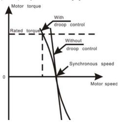
Figure 6.25 Droop control diagram
