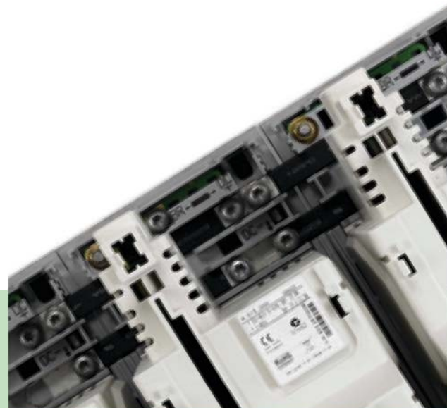
Common DC bus configuration enables braking energy to be recycled within the drive system
